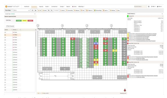
Health and Capacity Map provides an easy to understand status view of your data center Power, Current, Temperature, Humidity, Airflow, Pressure and more.
