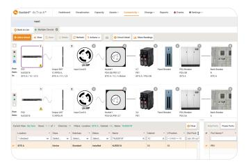
dcTrack Connection Management provides the ability to budget power at every connection point from the UPS to the power supply with (n) or (N+1) redundancy.
