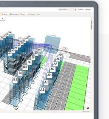
Measure distances between items so you'll always have just the right length of cabling. See cable tray layers for fiber, copper, and other cable
